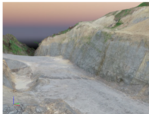
3d representation of Puture stockpile where volume calculations can be made
