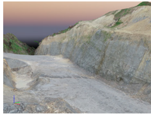
3d representation of Puture stockpile where volume calculations can be made
