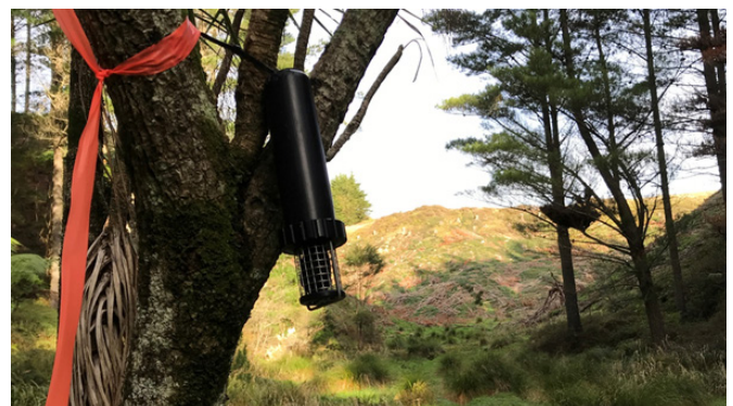
Figure 2. An ABM deployed in a wetland to record the presence of bat echolocation and kiwi calls.
