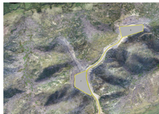
An example of using orthophotos to check the alignment of roads and skids
