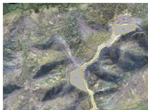
An example of using orthophotos to check the alignment of roads and skids
