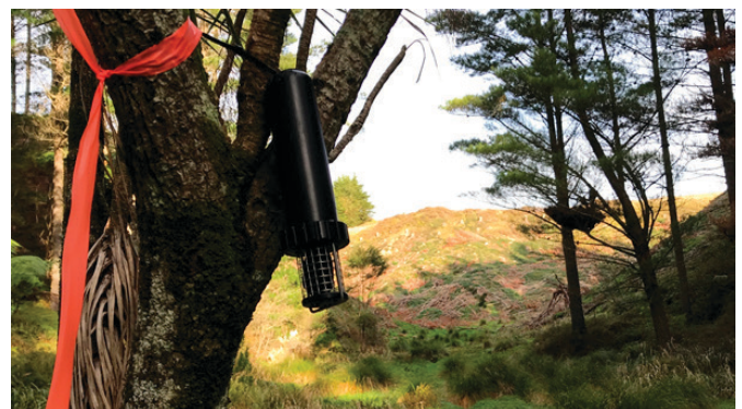
Figure 1. An ABM deployed in a wetland to record the presence of bat echolocation and kiwi calls.
