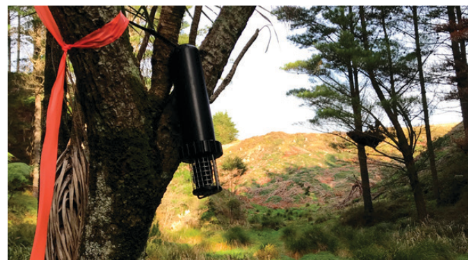
Figure 1. An ABM deployed in a wetland to record the presence of bat echolocation and kiwi
