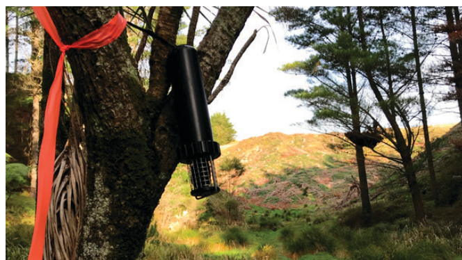
Figure 1. An ABM deployed in a wetland to record the presence of bat echolocation and kiwi
