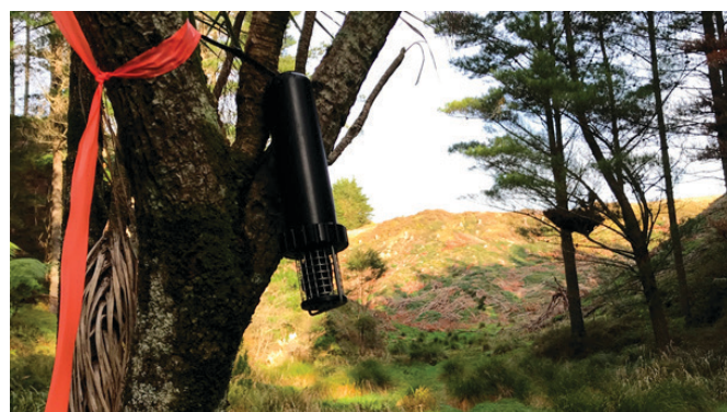
Figure 1. An ABM deployed in a wetland to record the presence of bat echolocation and kiwi calls.
