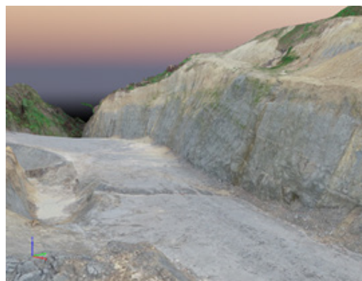
3d representation of Future stockpile where volume calculations can be made
