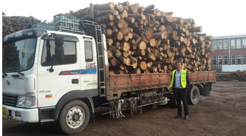
Will beside a load of Korean pine for chipping. Note the logs are stacked across the truck - less tha 2.4m long.
