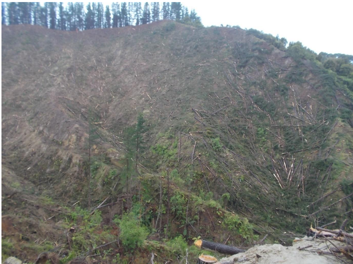
Figure 8: Skid 54's setting - note the standing trees with wind throw through them on the steep centre ridge. This was left by the faller with the standing trees and wind thrown stems grapple hauled to the skid where they were processed safely. Having the capacity with a swing yarder to grapple the stems makes it much safer for the crew in these situations.
