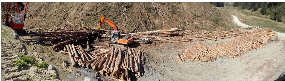
Figure1: Madil hauler extracting stems from setting 26a, Waikare Rd (Landing 45).
